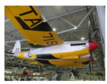
In the Airspace hanger we had a talk about the Mosquito, a small aircraft constructed mainly from wood. This was not seen as a viable option at first but improvements led to
